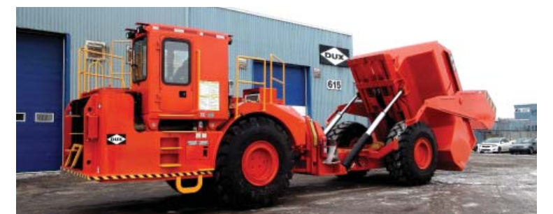
DUX TD-50 shown with front box section positioned ahead of rear section.
